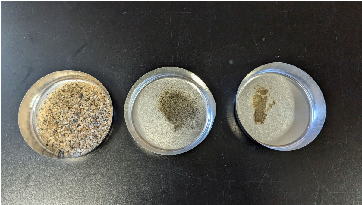
Figure 3: Fractionation of the suspended sediments <2\text{mm} collected during stormflow at Patapsco River site. Left 2-0.2 mm fraction, middle 0.2-0.06 mm fraction, right <0.06\text{ mm} .
