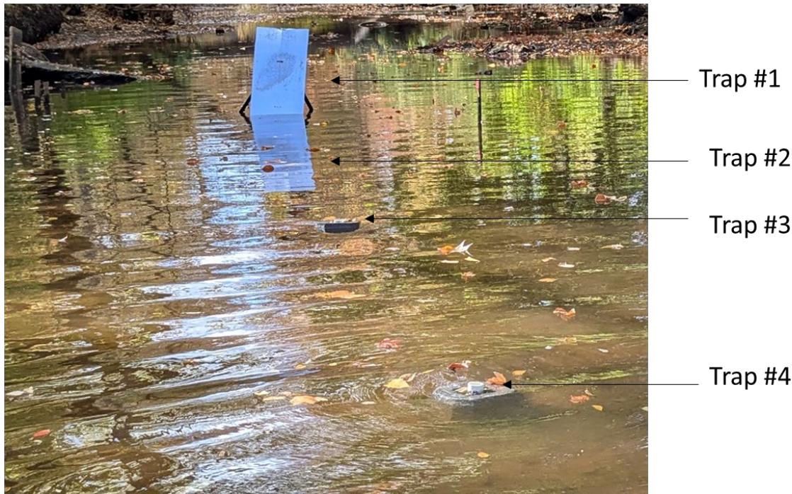
Figure 5: Sediment traps deployed at LBC1
