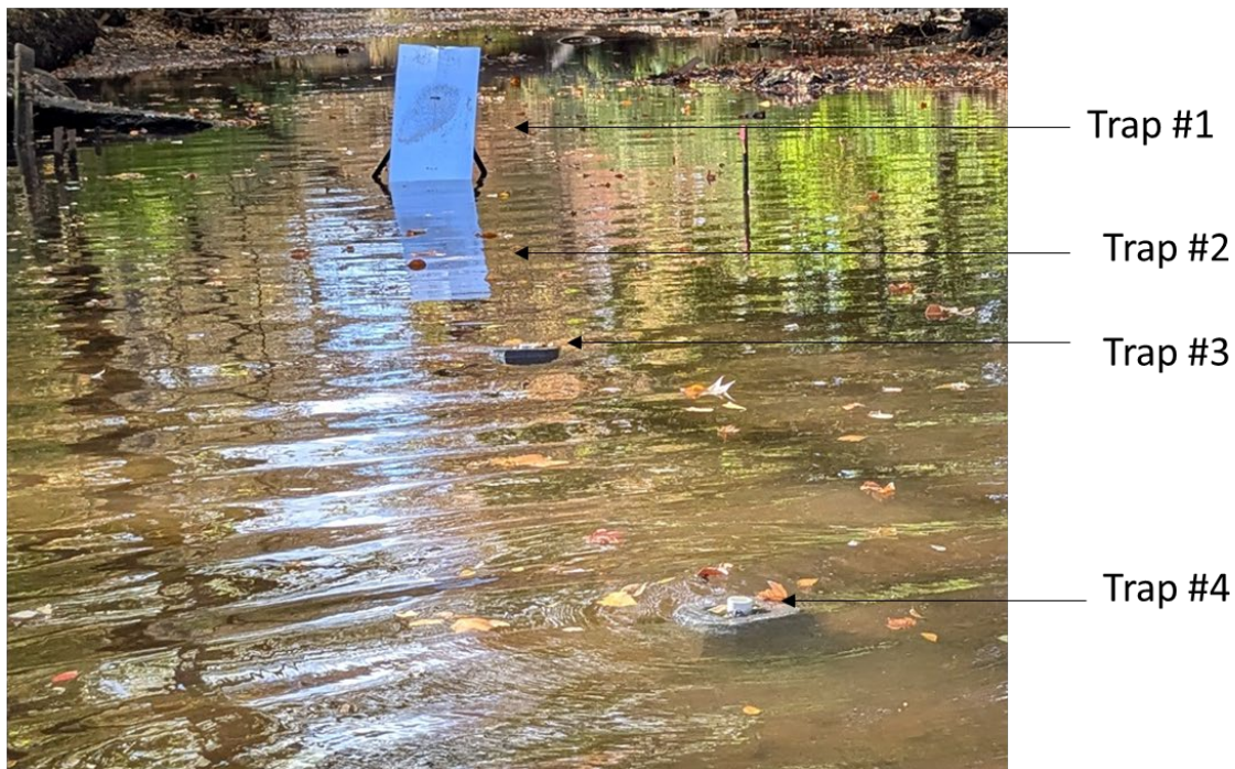
Figure 5: Sediment traps deployed at LBC1
