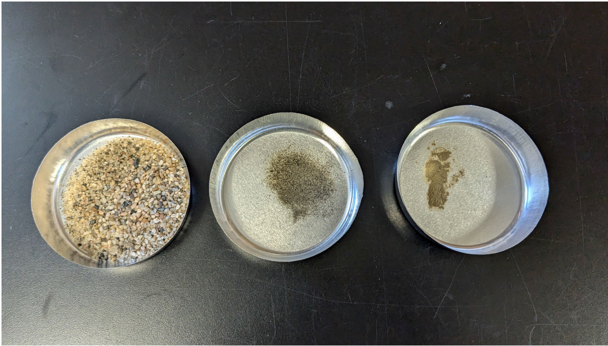
Figure 3: Fractionation of the suspended sediments <2mm collected during stormflow at Patapsco River site. Left 2-0.2 mm fraction, middle 0.2-0.06 mm fraction, right <0.06 mm.
