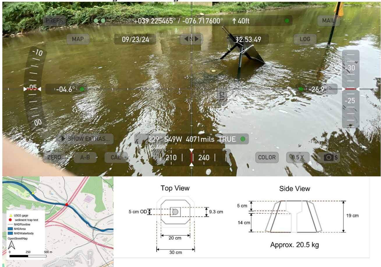
Figure 1: Sediment trap test in the Patapsco River. Top picture: Overall setting of the sediment trap and baffle in the Patapsco River. Bottom left: map of the sediment trap location. Bottom right: sediment trap design.
