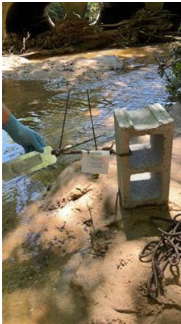
Figure 1. Example of surface water sampling apparatus used to support sampling media for PCB sampling.
