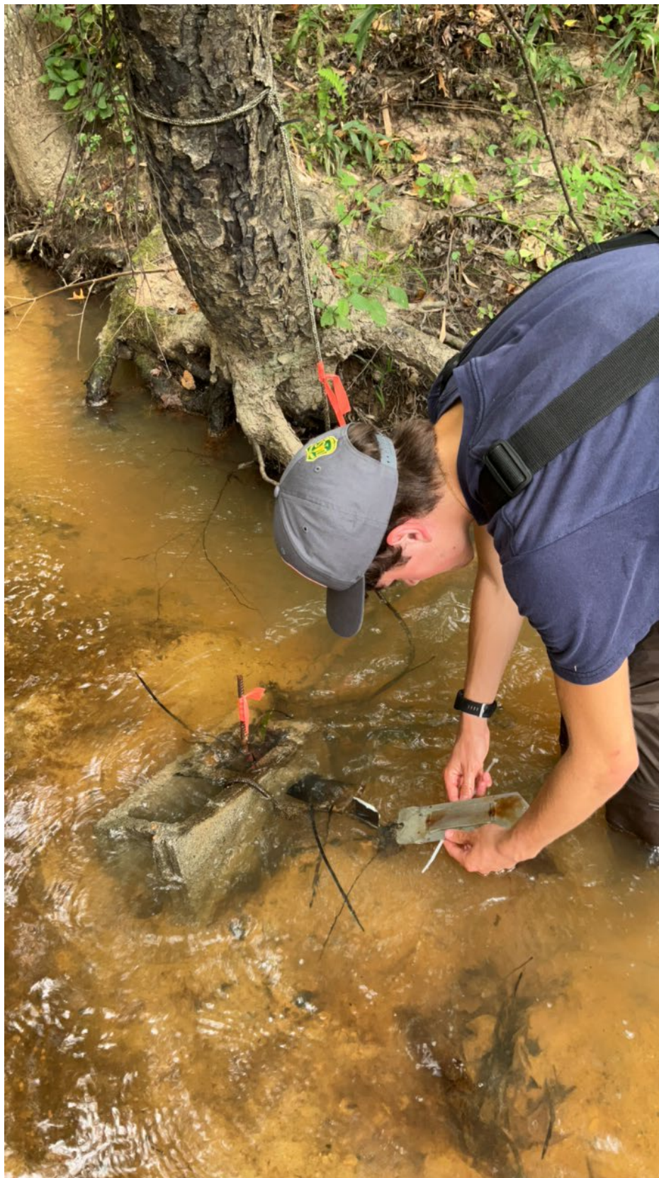
Figure 2. Repairs being made to surface water sampling device during a 30-day check.
